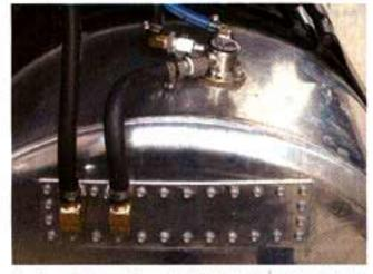
On Great Lakes Brewing Co.'s International delivery truck, the saddle tank is modified to handle SVO. The plate covers an opening that was cut to allow installation of a large transmission fluid
