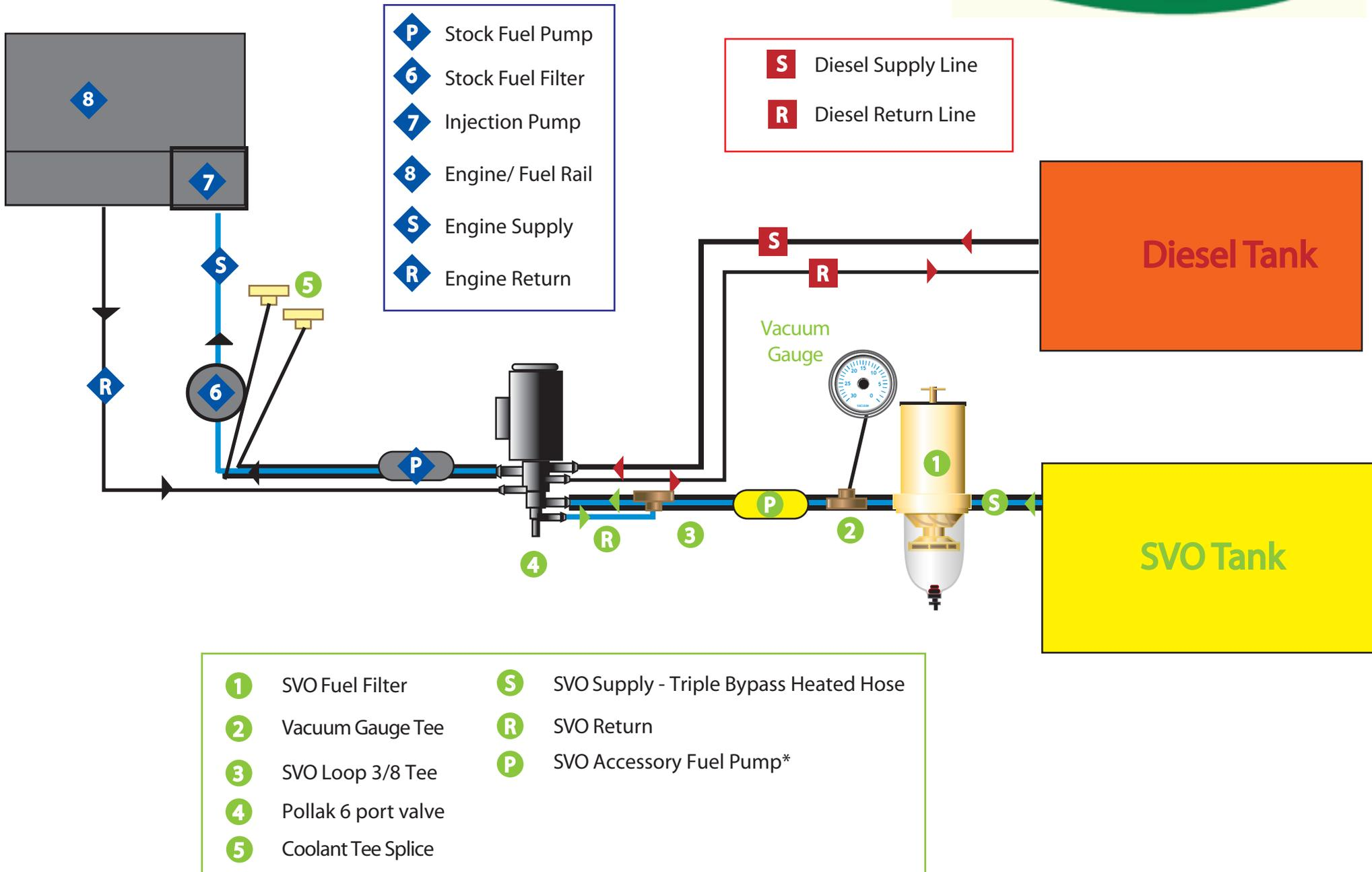
\*The SVO Fuel Pump must be wired to the switch so it is activated while running SVO and deactivated when running diesel.
