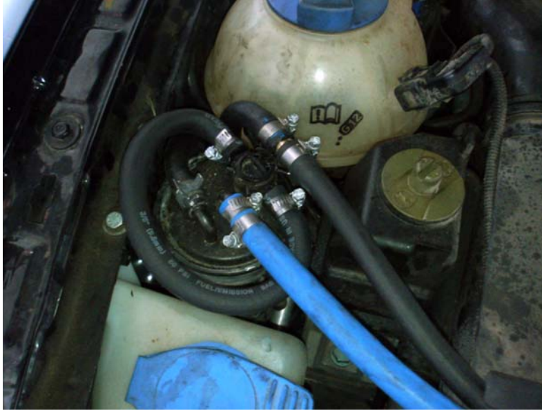
VW Stock Filter with Thermostatically Controlled Valve Bypassed – Note the Loop
