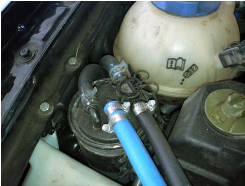
VW Stock Filter with Thermostatically Controlled Valve Not Bypassed
