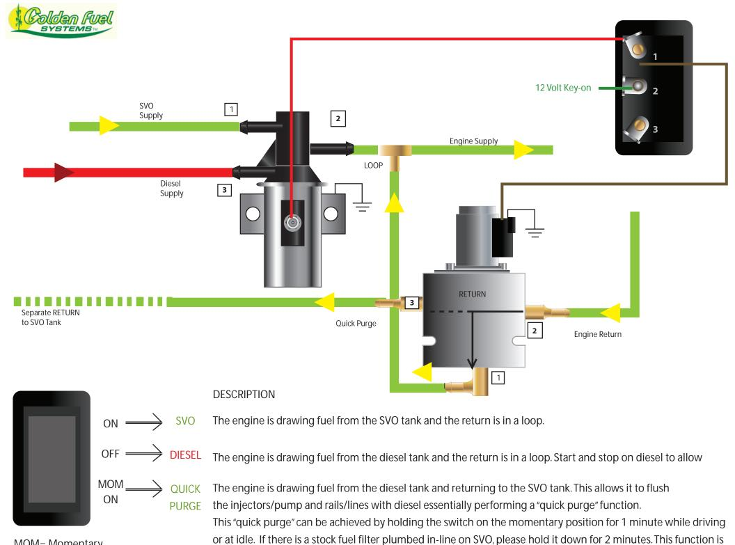
also useful to purge air out of either diesel or svo system.
