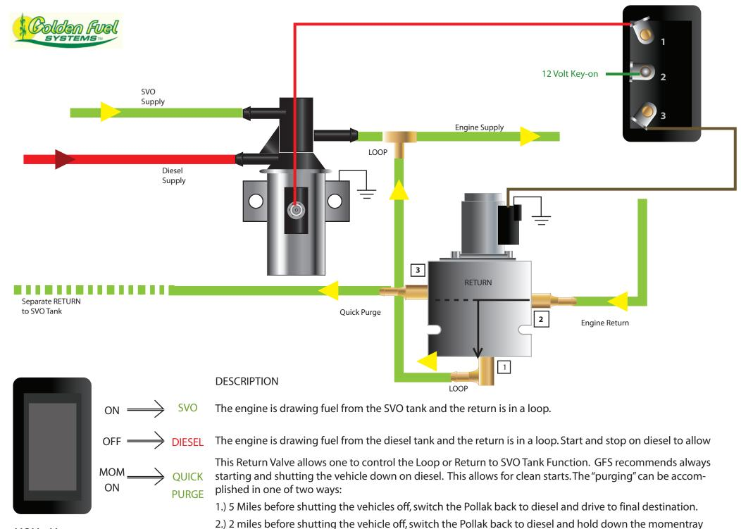
toggle switch until you turn the vehicle off. The Momentary toggle switch can be held down while at an idle, as well. If there is a stock fuel filter plumbed in-line on SVO, please hold the momentary toggle switch down for 3
